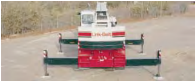
Fully Extended Outriggers 20' 6" (6.25 m) Spread
