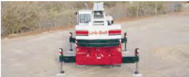
Intermediate Outriggers 14' 2" (4.32 m) Spread
