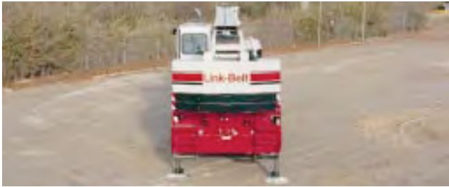
Retracted Outriggers 7' 9" (2.36 m) Spread
