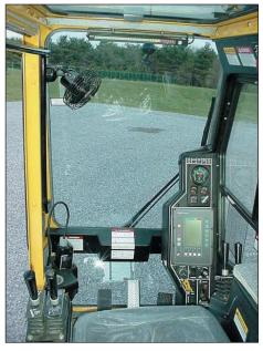
All steel fabricated superstructure cab has padded acoustical lining for sound suppression, safety glass and excellent visibility under close working conditions.
